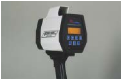
Laser guns are aimed with a sight, like a rifle.
