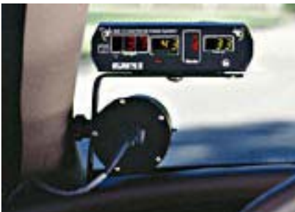
Radar units send a wide beam that tracks all vehicles within range without precise aiming.
